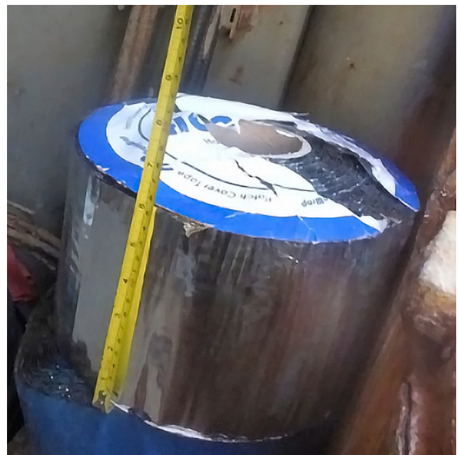
Figure 16: Hatch cover sealing tape
