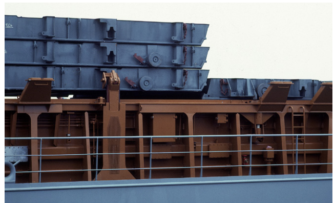
Figure 9: Stacking hatch covers
