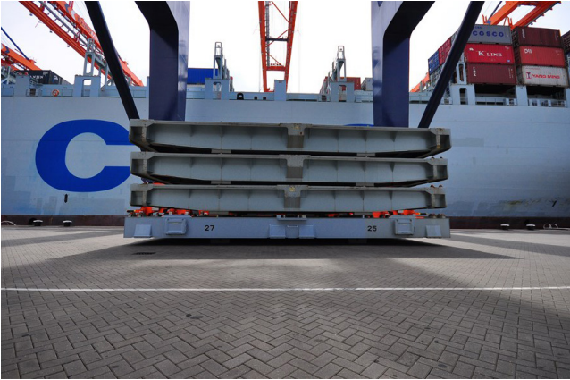
Figure 6: Lift-away (pontoon) hatches
