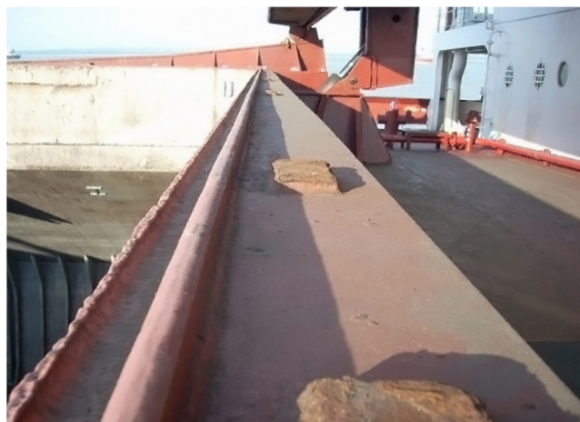
Figure 35: Compression bar – straight, undamaged and non-corroded
